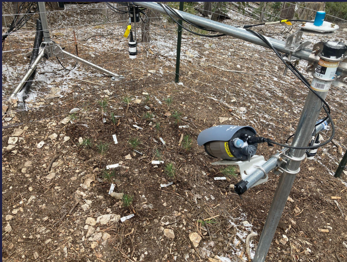
Photo of instrumentation used to monitor planted seedling survival at HTNF. This site is in Scout canyon, near the existing SNOTEL station.
